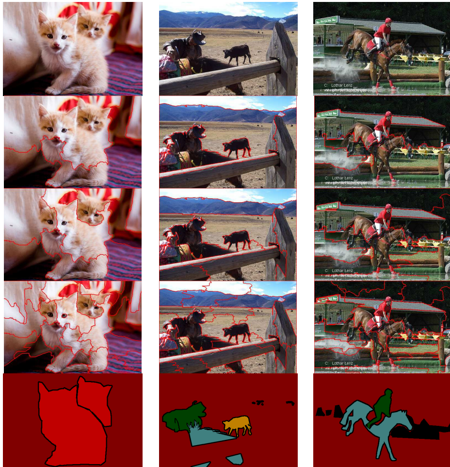
Figure 1.4: Example multi-scale segmentations from the VOC 2008 dataset. Rows one to four: Image segmentation at progressively finer levels of detail. Bottom row: Pixel-level class labels.
