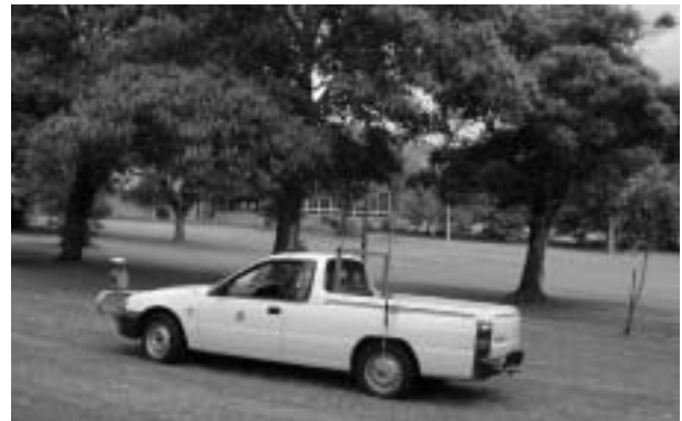
Fig. 8. The vehicle used in our experiments is equipped with a two-dimensional laser range finder and a differential GPS system. The vehicle's ego-motion is measured by a linear variable differential transformer sensor for the steering, and a wheel-mounted velocity encoder. In the background, the Victoria Park test environment can be seen.
