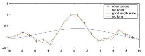
The mean posterior predictive function is plotted for 3 different length scales (the green curve corresponds to optimizing the marginal likelihood). Notice, that an almost exact fit to the data can be achieved by reducing the length scale – but the marginal likelihood does not favour this!
