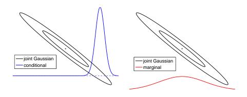
Both the conditionals and the marginals of a joint Gaussian are again Gaussian.
